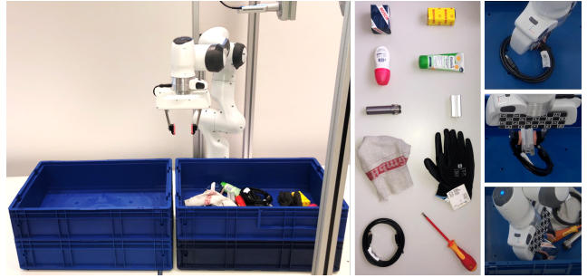
Fig. 6: Experimental setup with robotic arm, parallel-jaw gripper, overhead RGBD camera and bins (left), diverse object portfolio (middle), successful grasp (top right), failure grasp (middle right), collision grasp (bottom right).
