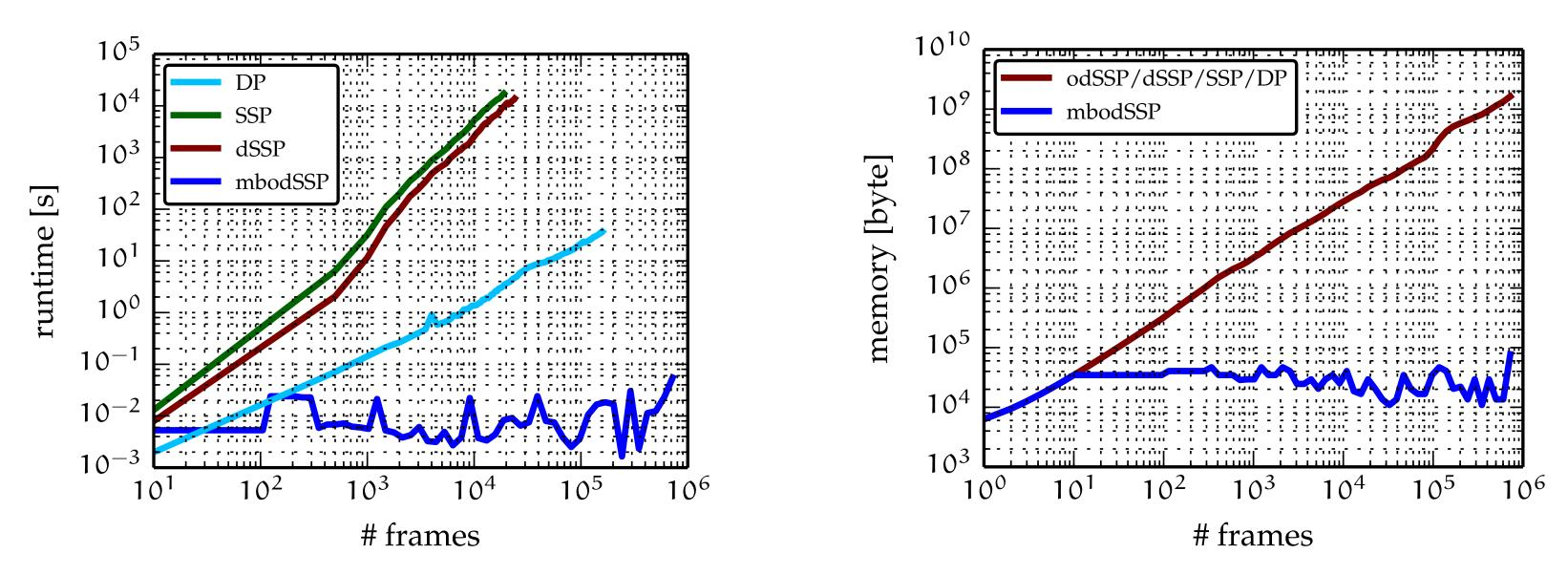
Run Time and Memory Comparison. Computational performance of all solvers using one long sequence. From left to right: Mean runtime and idealized memory consumption for every solver.
