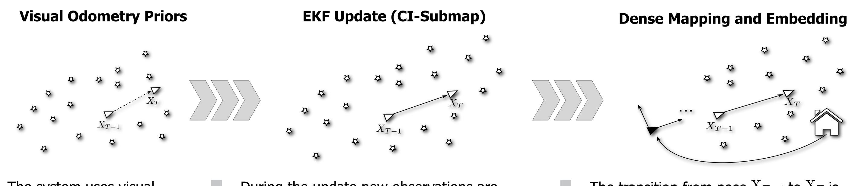
The system uses visual odometry prirors to predict the state vector of the sparse SLAM estimate. This includes the current robot pose. As VO the method of Kaess et al. 2009 is used.
