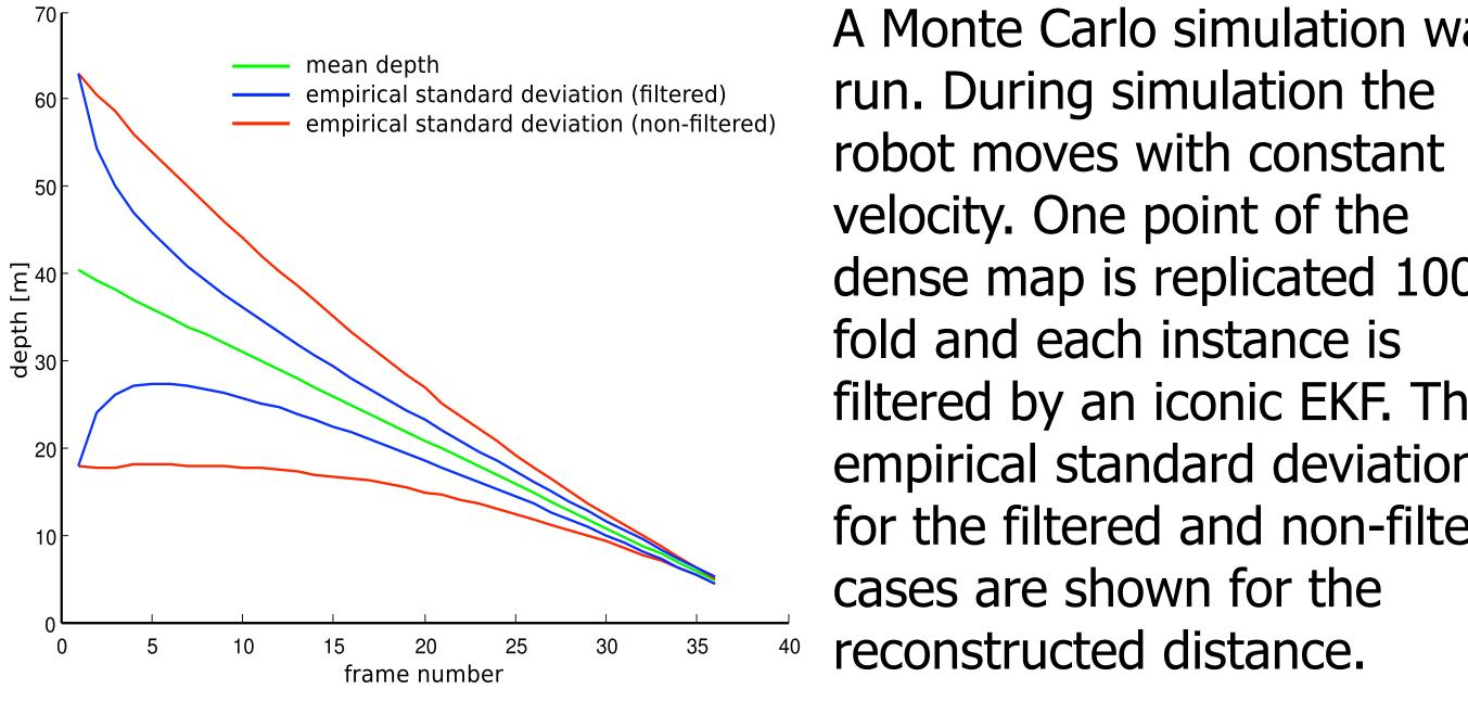
A Monte Carlo simulation was dense map is replicated 1000filtered by an iconic EKF. The empirical standard deviations for the filtered and non-filtered
