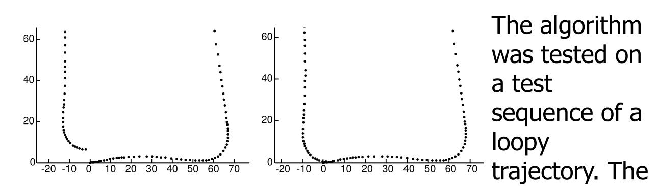
car like robot moved with speeds of up to 30 km/h. The drift before closing the loop (shown above) is approximately 5m. After closing the loop drift is resolved. The bottom shows the dense map associated with that trajectory. It can be seen how the dense maps align well after loop closure. Loop closure was triggered manually.
