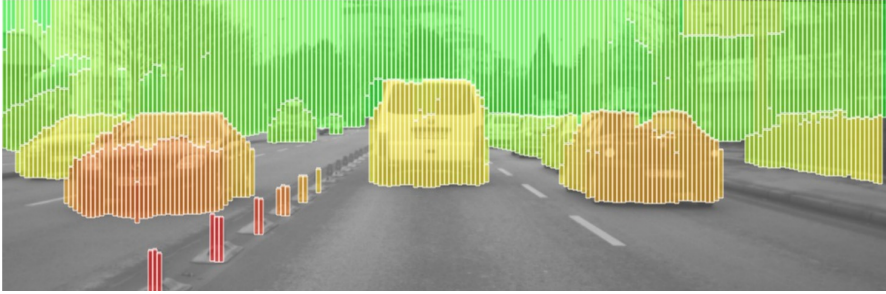
Figure 7.10: Multi-layer Stixel World. The multi-layer Stixel World representation of Pfeiffer and Franke [511]. The scene is segmented into planar segments termed “Stixels”. In contrast to the Stixel World of [21], objects are allowed to be located at multiple depths within a single image column. The color represents the distance to the obstacle with red being close and green far away. Figure courtesy of Pfeiffer and Franke [511] © 2016 BMVA.
