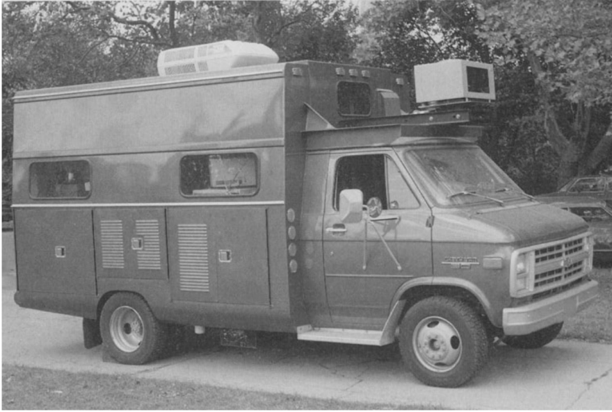
Figure 2.1: The Navlab. The self-contained laboratory from CMU for navigational vision system research. Figure courtesy of Thorpe et al. [649] © 1988 Springer.
