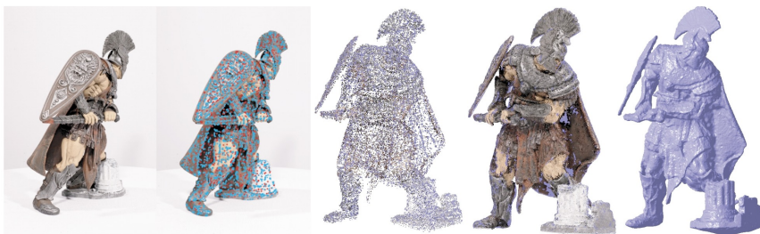
Figure 10.2: Point Cloud and Surface Representation. The different steps of Patch-based Multi-View Stereo (PMVS) [217]. The input image, extracted features, reconstructed patches from the initial matching, reconstruction after expansion and filtering, and the final polygonal surface representation. Figure courtesy of Furukawa and Ponce [217] © 2010 IEEE.
