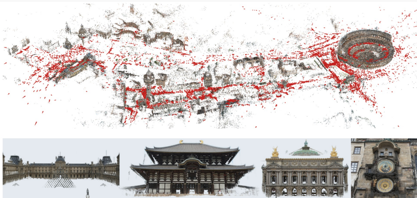
Figure 10.1: Large-Scale 3D Reconstruction. Upper row: Coarse reconstruction and camera pose estimation (red) from the SfM [588] pipeline of COLMAP. Bottom row: Fine reconstruction with the MVS [589] pipeline of COLMAP. Figure courtesy of Schönberger and Frahm [588] and Schönberger et al. [589] © 2016 IEEE.
