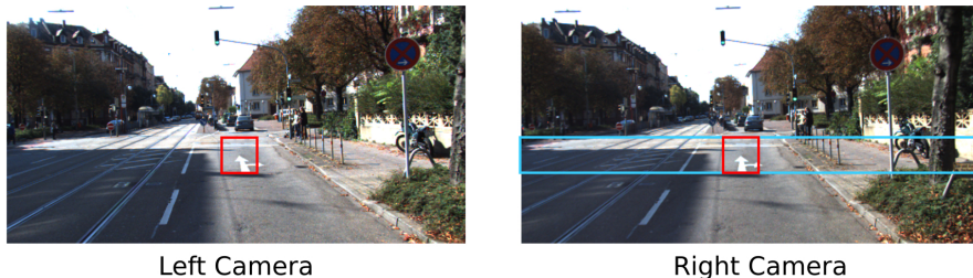
Figure 9.1: Stereo Matching Problem. Visualization of the stereo matching problem. Given two rectified images (from KITTI training [238]), stereo matching reduces to a 1D search problem along the epipolar line (blue rectangle).
