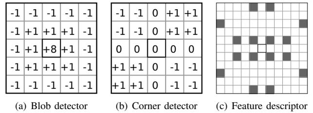
Fig. 3. **Blob/corner detector and feature descriptor:** Our feature detections are minima and maxima of blob and corner filter responses. The descriptor concatenates Sobel filter responses using the layout given in (c).
