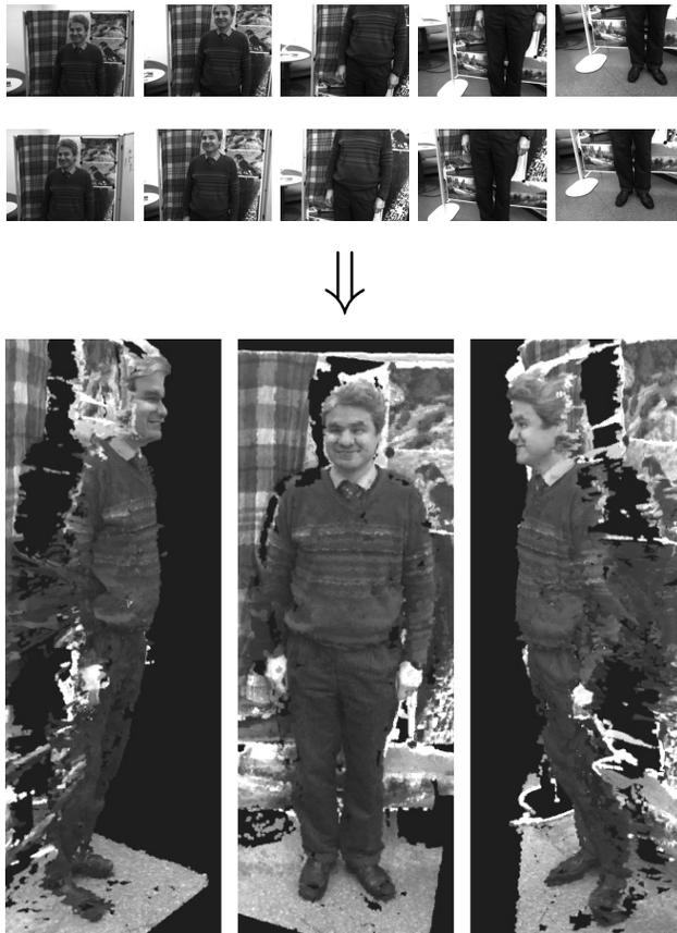
Fig. 1. **Real-time 3d reconstruction based on stereo sequences:** Our system takes stereo images (top) as input and outputs an accurate 3d model (bottom) in real-time. All processing is done on a single CPU.
