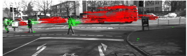
(b) Feature tracking (5 frames, static camera)
