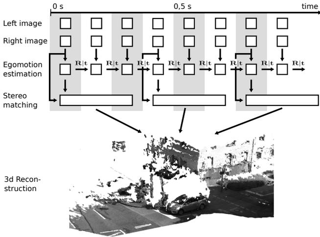
Fig. 2. **System overview:** We use two worker threads in order to obtain egomotion estimates and disparity maps in parallel: While the stereo matching and 3d reconstruction part runs at 3-4 fps (Sec. III C+D), our sparse feature matching and visual odometry system (Sec. III A+B) achieves 25 fps. Taken together, this is sufficient for online 3d reconstruction.
