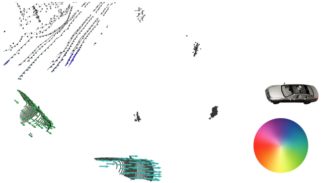
Figure 1: Scene Flow Prediction by SLIM. Flow vectors are colored by their direction and magnitude as illustrated with the color wheel. Our method correctly annotates the background as static and produces consistent results for the two vehicles, matching the ground truth scene flow.
