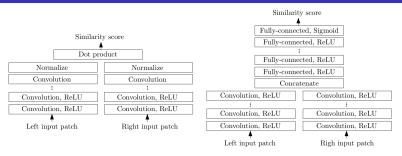
Matching cost computation by learning a similarity measure on patches using a CNN
