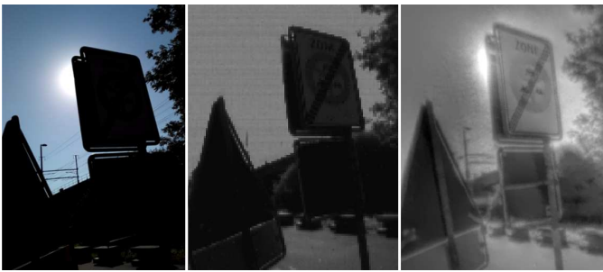
Fig. 12: Outdoor sequence, pointing at the sun. Left: View from a standard camera, showing severe under-exposure on the foreground. Middle: Frame from the DAVIS, showing severe under- and over-exposed areas. Right: HDR image reconstructed using the output of EVO.
