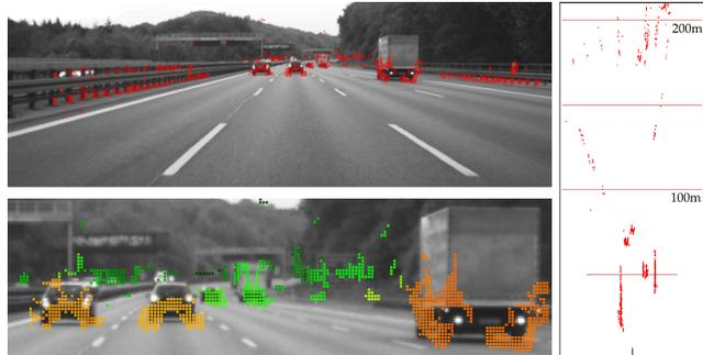
Fig. 1. Example of obstacles detected by the proposed system at distances between 50 and 200 m (top, red), close-up of the resulting distance estimates (red: close, green: far) and corresponding bird's eye view (right)
