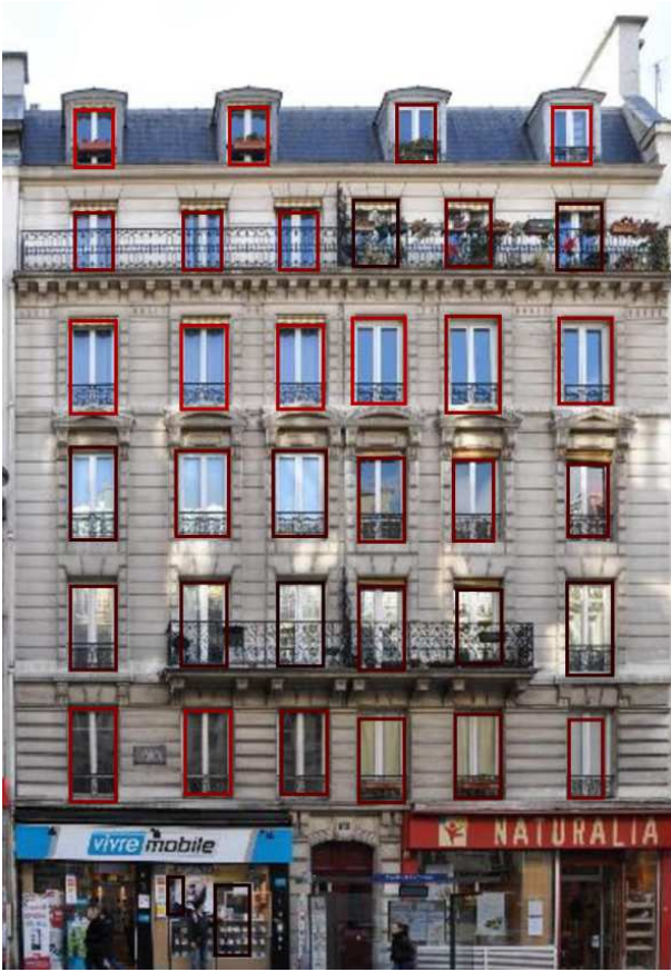
Fig. 7 Example detections of the Very Fast specific window detector. The color encodes the confidence of the detection from high confidence (red) to low confidence (black).
