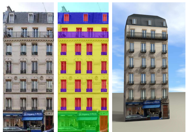
Fig. 1 The input to our system is cropped and rectified facade image (left). We process the image by our three layers to produced a labeled output image (middle). From this output we produce a textured procedural model (right).
