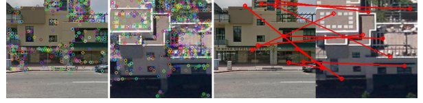
Figure 4: Key points matching fails on aerial-to-ground view image pairs for our problem.
