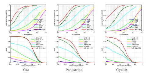
**Fig. 6.** Proposal performance comparison on KITTI validation set (moderate). The first row is proposal recall curves and the second row is recall v.s. *IoU* for 100 proposals.
