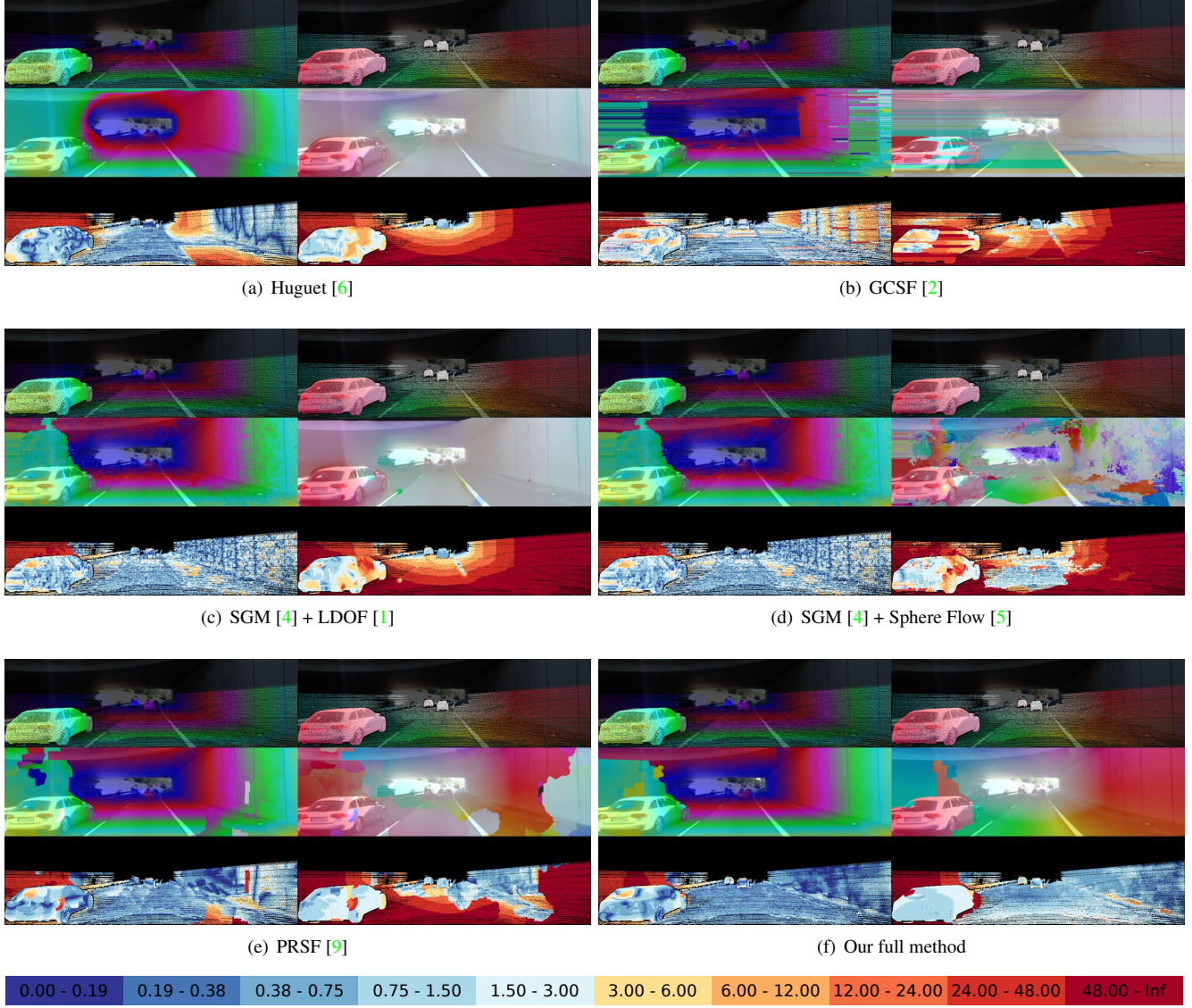
Figure 34: Comparison of Results. Each subfigure shows from top-to-bottom: The disparity and optical flow ground truth in the reference view, the disparity map (D1) and optical flow map (FI) estimated by the specified algorithm, and the respective error images using the color scheme depicted in the legend.
