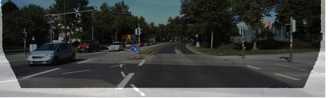
Figure 2: Visibility Mask. Image regions visible in the first frame but not in the second frame are shown in white.
