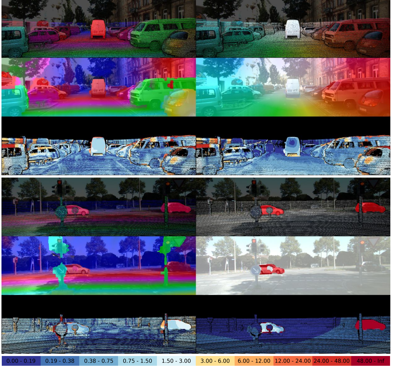
Figure 7: Qualitative Results. Each subfigure shows from top-to-bottom: The disparity and optical flow ground truth in the reference view, the disparity map (D1) and optical flow map (F1) estimated by our scene flow algorithm, and the respective error images using the color scheme depicted in the legend.
