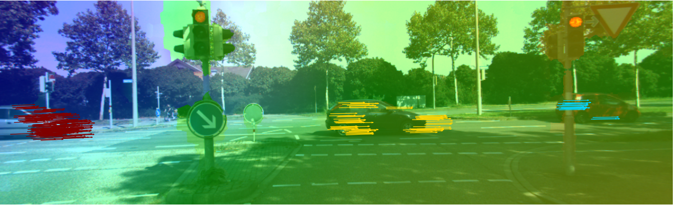
Figure 3: Object Hypotheses Generation. This figure depicts the optical flow field induced by the camera motion and the remaining sparse scene flow features grouped into individual motion hypotheses using color-coded flow vectors.
