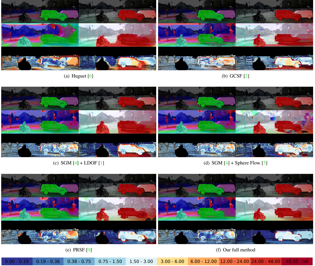
Figure 31: Comparison of Results. Each subfigure shows from top-to-bottom: The disparity and optical flow ground truth in the reference view, the disparity map (D1) and optical flow map (F1) estimated by the specified algorithm, and the respective error images using the color scheme depicted in the legend.
