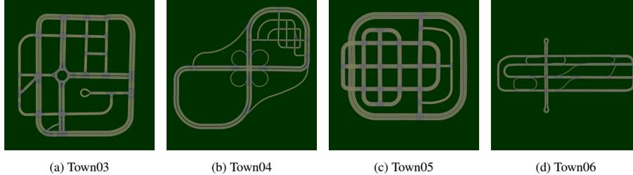
Fig. 2: **Town layouts.** Each town has unique features, such as roundabouts (a) or highway junctions (b, d).
