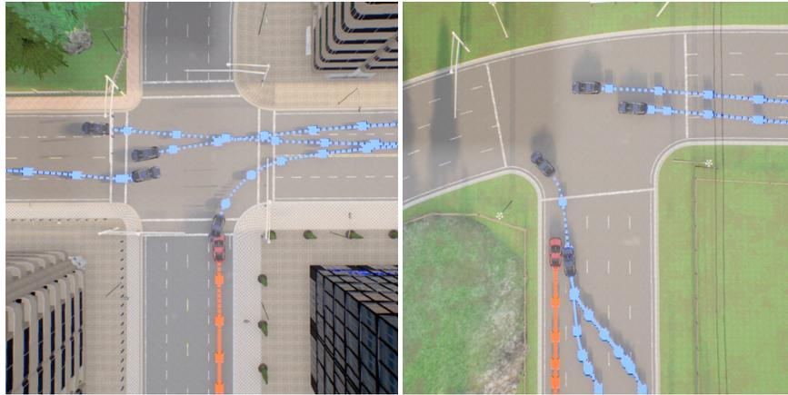
Fig. 11: **KING failure cases.** As we aim to cover the long tail of the distribution of traffic scenarios, we impose few constraints on the trajectories of other traffic participants. This can lead to unlikely behaviour in the background actors by definition, such as moving into opposing lanes (left) or performing seemingly unnecessary lane changes (right).
