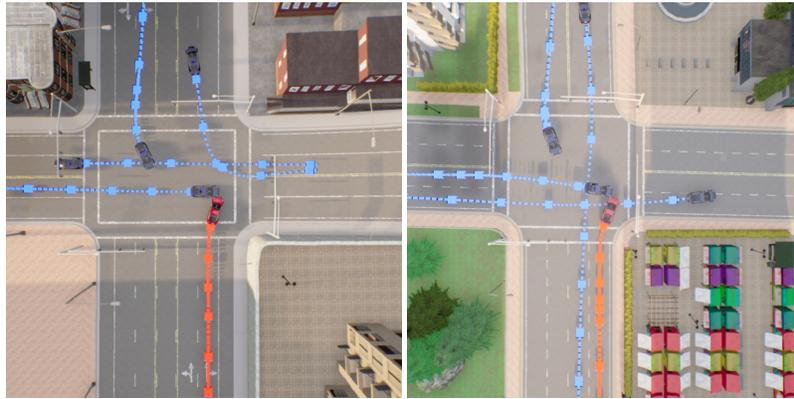
Fig. 8: AIM-BEV - Cluster (e). The driving agent fails to brake when traffic in the intersection does not yield. As a result the agent collides into the side of another vehicle.
