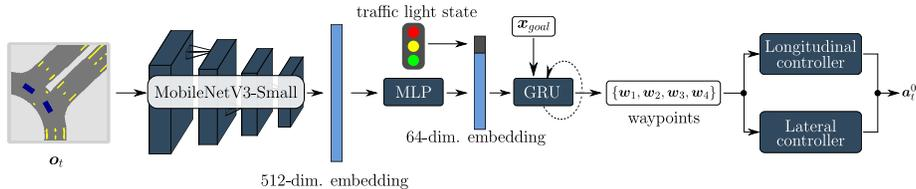
Fig. 1: **Architecture Overview.** Illustration of the AIM-BEV architecture. First, a low-dimensional embedding from the input BEV semantic grid map observation  $\mathbf{o}_t$  is extracted. This is then used as the basis for autoregressive waypoint prediction, from which the final actions are obtained via lateral and longitudinal PID controllers.
