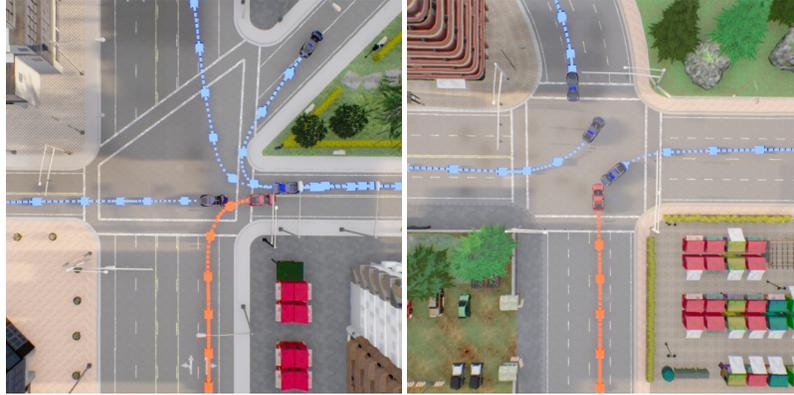
Fig. 5: AIM-BEV - Cluster (b). The driving agent understeers when taking a turn, colliding with another vehicle that has been slightly displaced from its lane center by the safety-critical perturbation (left). Background traffic in CARLA usually closely adheres to the lane centers, making penalization of bad lane following less likely. On the right hand side, overconfident behavior in an unprotected intersection leads to collision.
