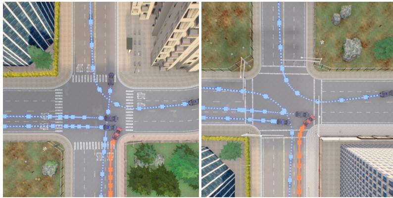
Fig. 9: AIM-BEV - Cluster (f). The examples shown here depict similar situations as in cluster (e). The ego agent fails to correctly assess if it is safe to continue on, resulting in other traffic colliding into its side.
