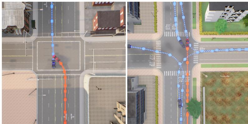
Fig. 7: **AIM-BEV - Cluster (d)**. This cluster primarily features collisions at the side of the driving agent. As depicted, this type of collision can arise from insufficient safety distance while turning (left) or failure to yield for another vehicle taking an aggressive turn (right).
