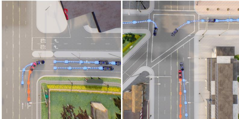
Fig. 4: AIM-BEV - Cluster (a). The driving agent collides with a slow moving vehicle while taking a turn (left). Additionally, it often struggles to handle lane-change scenarios safely (right). This is also evident in cluster (c).
