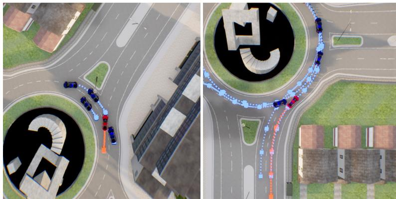
Fig. 6: AIM-BEV - Cluster (c). The driving agent fails to handle merges and lane-changes in a roundabout safely. These maneuvers are especially problematic due to AIM-BEV's forward facing field of view. This shortcoming is not as apparent in regular CARLA traffic, highlighting KING's ability to draw attention to possible failure modes.
