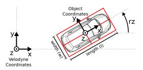
Fig. 7. **Object Coordinates.** This figure illustrates the coordinate system of the annotated 3D bounding boxes with respect to the coordinate system of the 3D Velodyne laser scanner. In *z*-direction, the object coordinate system is located at the bottom of the object (contact point with the supporting surface).
