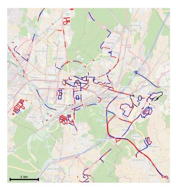
Fig. 2. **Recording Zone.** This figure shows the GPS traces of our recordings in the metropolitan area of Karlsruhe, Germany. Colors encode the GPS signal quality: Red tracks have been recorded with highest precision using RTK corrections, blue denotes the absence of correction signals. The black runs have been excluded from our data set as no GPS signal has been available.
