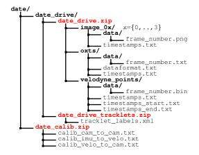
Fig. 4. Structure of the provided Zip-Files and their location within a global file structure that stores all KITTI sequences. Here, 'date' and 'drive' are placeholders, and 'image\_0x' refers to the 4 video camera streams.
