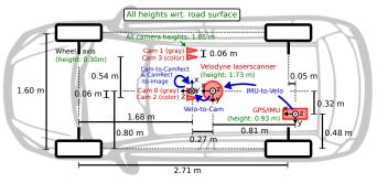
Fig. 3. **Sensor Setup.** This figure illustrates the dimensions and mounting positions of the sensors (red) with respect to the vehicle body. Heights above ground are marked in green and measured with respect to the road surface. Transformations between sensors are shown in blue.
