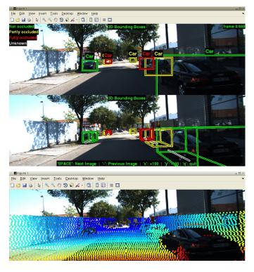
Fig. 6. **Development kit.** Working with tracklets (top), Velodyne point clouds (bottom) and their projections onto the image plane is demonstrated in the MATLAB development kit which is available from the KITTI website.
