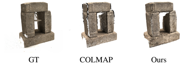
Figure 12: Example reconstructed cloud for an element of the test set. Note the significant imperfections in the reference point cloud (left). A visual drawback of our approach is that we focus solely on structure; the fusion step used by COLMAP innately also averages out the difference in color appearance between various views.
