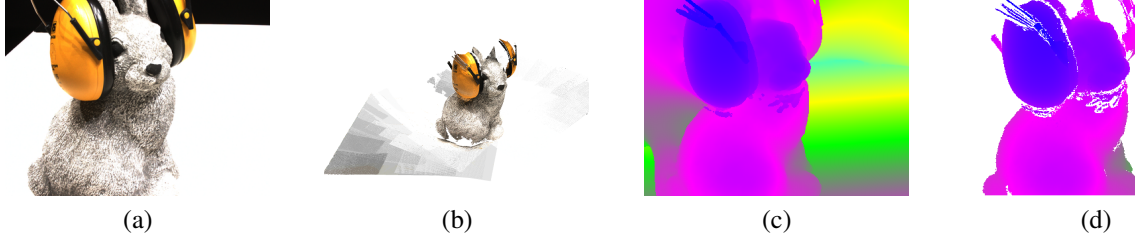
Figure 8: The depth maps used for supervision on the DTU dataset. For a given input image (a), the dataset contains a reference point cloud (b) obtained with a structured light scanner. After creating a watertight mesh (c) from this point cloud and projecting that, we reject any point in the point cloud which gets projected behind this surface from the supervision depth map (d). Additionally, we reject the points of the white table.
