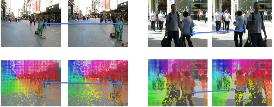
Fig. 2: Visualization of the DeepMatching results on the MOT16 sequences
