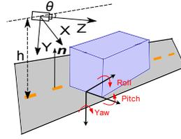
Figure 2. Geometry of ground plane estimation and object localization. The camera height  $h$  is the distance from its principal point to the ground plane. The pitch angle is  $\theta$  and  $\mathbf{n}$  is the ground plane normal. Thus, the ground plane is defined by  $(\mathbf{n}^\top, h)^\top$ .
