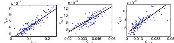
Figure 5. Fitting a model  $\mathcal{C}_s$  to relate observation variance  $v_s$  to the belief in accuracy  $\mathbf{c}_s$  of dense stereo, for  $h$ ,  $n_1$  and  $n_3$ .
