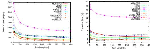
Figure 11. Comparison with other SFM systems. Our system is labeled MLM-SFM, shown in solid red. Note that we nearly match even state-of-the-art stereo for rotation and compete well against stereo in translation as well. Note the wide improvement over other monocular systems. See KITTI webpage for complete details.
