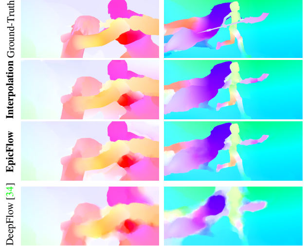
Figure 7. From top to bottom : ground-truth flow, result of sparse-to-dense interpolation (Interpolation), full method (EpicFlow), and DeepFlow [34], one of the top performers on MPI-Sintel.
