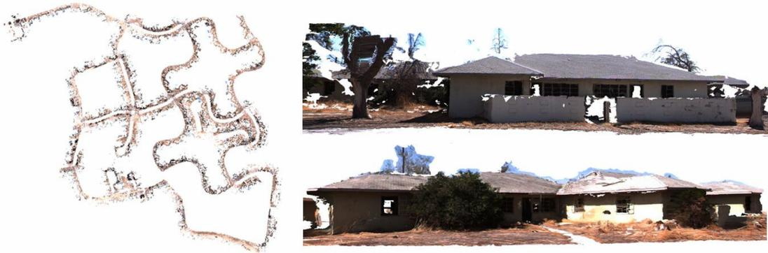
Figure 1: View from above and details of reconstructed models from a 170,000 frame video
