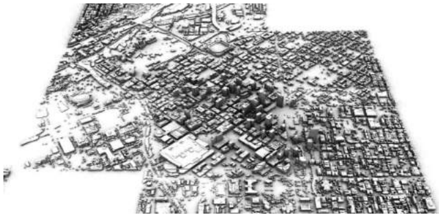
Figure 29: Large scale reconstruction of Downtown Denver and surrounding areas. The model is a polygonal mesh generated from air-borne LiDAR data. Figure courtesy of Charalambos Poullis [PY09a]. ©2009 IEEE.
