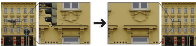
Figure 20: The input image on the left contains a traffic light and several cables. To the right the unwanted objects have been successfully removed by utilising the symmetry in the façade image [MWR*09].
