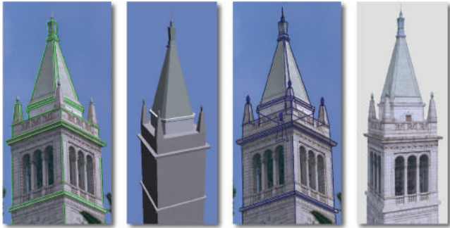
Figure 8: Interactive image-based modelling: (1) input image with user-drawn edges shown in green, (2) shaded 3D solid model, (3) geometric primitives overlaid onto the input image, (4) final view-dependent, texture-mapped 3D model. Figure courtesy of Paul Debevec [DTM96] ©1996 ACM.
