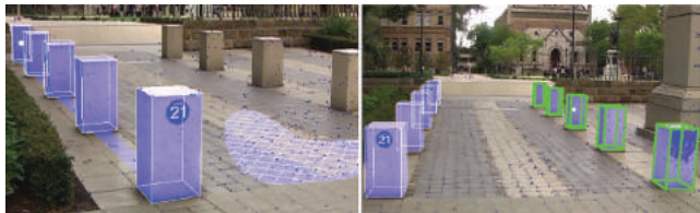
Figure 10: Interactive modelling of geometry in video. Left-hand side: Replicating the bollard by dragging the mouse. Right-hand side: Replicating a row of bollards. Figure courtesy of Anton van den Hengel [vdHDT*07a] ©2007 ACM.
