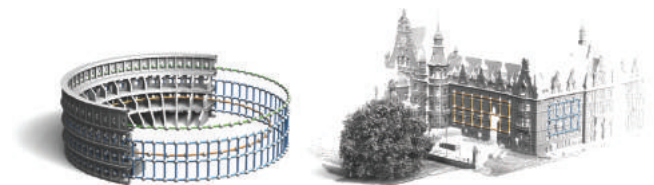
Figure 22: This example shows automatic symmetry detection results performed on point-clouds of architectural objects. Figure courtesy of Mark Pauly [PMW*08], ©2008 ACM.
