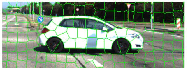
Figure 4. **Superpixels.** Typical oversegmentation of a car.
