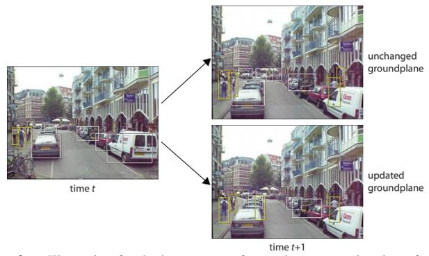
**Fig. 2.** Illustration for the importance of a continuous reestimation of scene geometry. The images show the effect on object detection when the vehicle hits a speedbump (top) if using an unchanged ground plane estimate; (bottom) if using the online reestimate.
