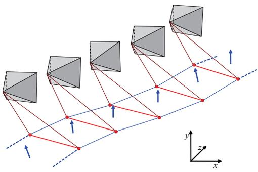
**Fig. 1.** Visualization of the online ground plane estimation procedure. Using the camera positions from SfM, we reconstruct trapezoidal road strips between the car’s wheel contact points of adjacent frames. A ground plane estimate is obtained by averaging the local normals over a spatial window of about 3m travel distance.
