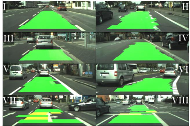
Fig. 10. Visualization of driving corridor results. Examples I-VI corresponding to Fig. 1. Green indicating *drivable* and yellow *narrow corridor*. The visualization is limited to a distance of 28m.
