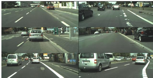
Fig. 1. Demo images showing the challenges in the urban dataset: Situations with bad lane-marking quality, curbstones as road delimiter, unmarked lanes, pot holes in the road and a strong curve.
