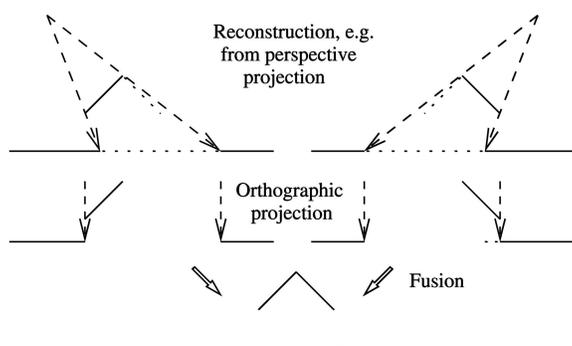
Fig. 8. Orthographic projection of disparity images and fusion.
