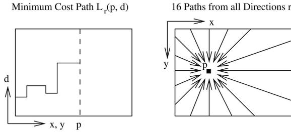
Fig. 2. Aggregation of costs in disparity space.
