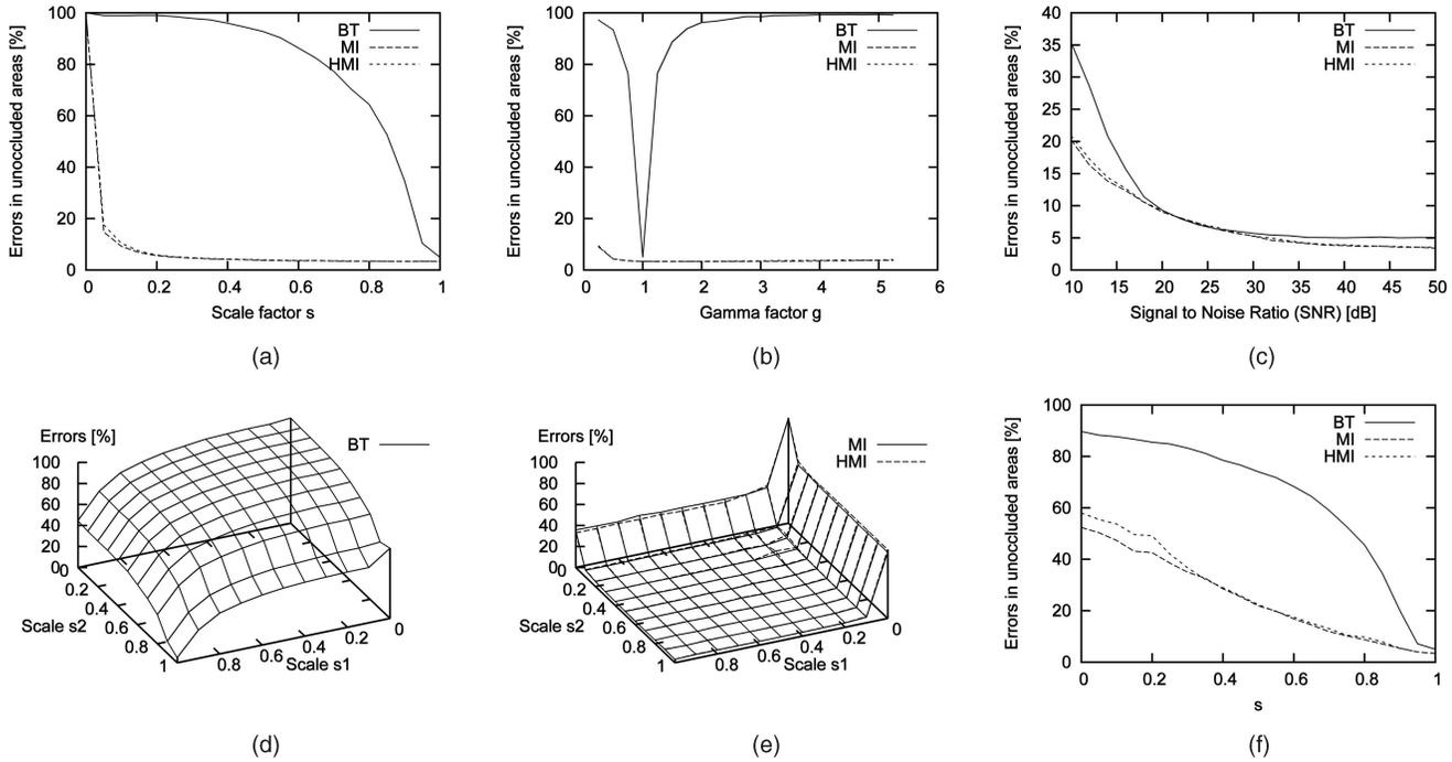
Fig. 10. Effect of applying radiometric changes or adding noise to the right match images using SGM with different matching cost calculations. (a) Global scale change, that is,  $I' = sI$ . (b) Global gamma change. (c) Adding Gaussian noise. (d) Different scaling of image halves. (e) Different scaling of image halves. (f) Linear down-scaling from center.
