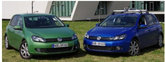
**Fig. 1:** The two test car platforms, each equipped with a set of four fish-eye cameras that provides an all-surround view of the environment.
