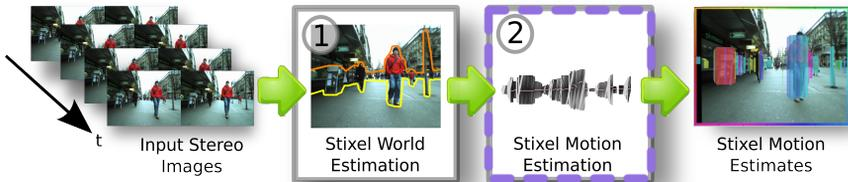
Figure 1: Pipeline of our motion estimation method. We focus on step 2.
