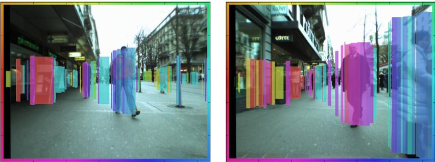
Figure 6: Example results of our stixel motion estimation algorithm. Motion vector orientation is colour coded (see image border). Left image shows frame 8.
