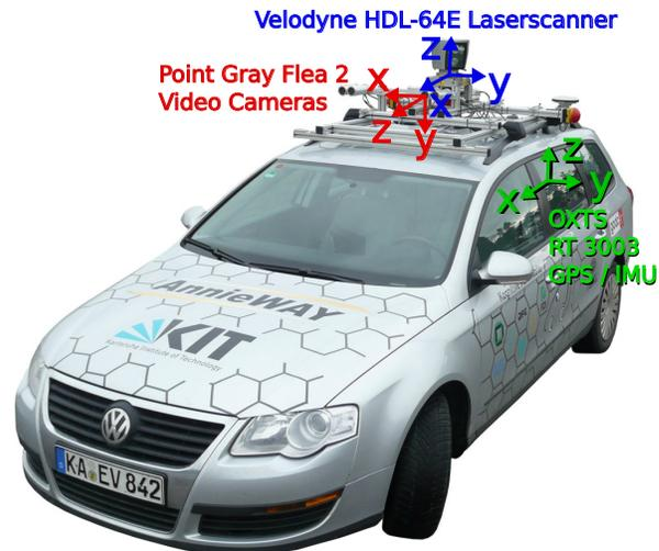
Fig. 1. **Recording Platform.** Our VW Passat station wagon is equipped with four video cameras (two color and two grayscale cameras), a rotating 3D laser scanner and a combined GPS/IMU inertial navigation system.
