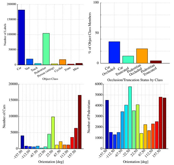
Fig. 8. **Object Occurrence and Orientation Statistics of our Dataset.** This figure shows the different types of objects occurring in our sequences (top) and the orientation histograms (bottom) for the two most predominant categories 'Car' and 'Pedestrian'.
