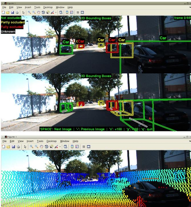
Fig. 6. **Development kit.** Working with tracklets (top), Velodyne point clouds (bottom) and their projections onto the image plane is demonstrated in the MATLAB development kit which is available from the KITTI website.
