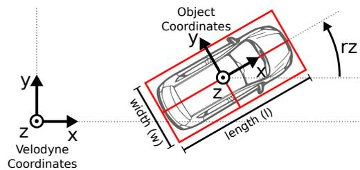
Fig. 7. **Object Coordinates.** This figure illustrates the coordinate system of the annotated 3D bounding boxes with respect to the coordinate system of the 3D Velodyne laser scanner. In  $z$ -direction, the object coordinate system is located at the bottom of the object (contact point with the supporting surface).
