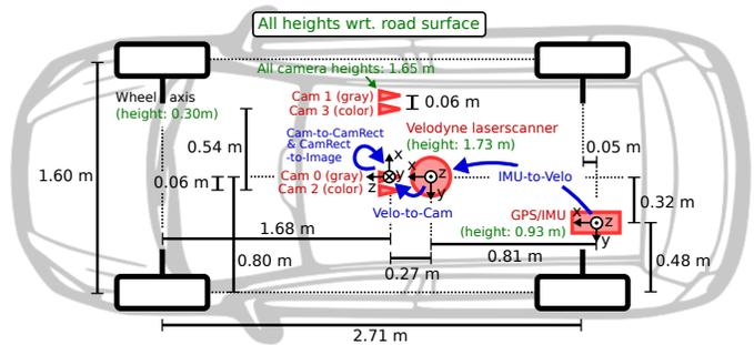
Fig. 3. **Sensor Setup.** This figure illustrates the dimensions and mounting positions of the sensors (red) with respect to the vehicle body. Heights above ground are marked in green and measured with respect to the road surface. Transformations between sensors are shown in blue.
