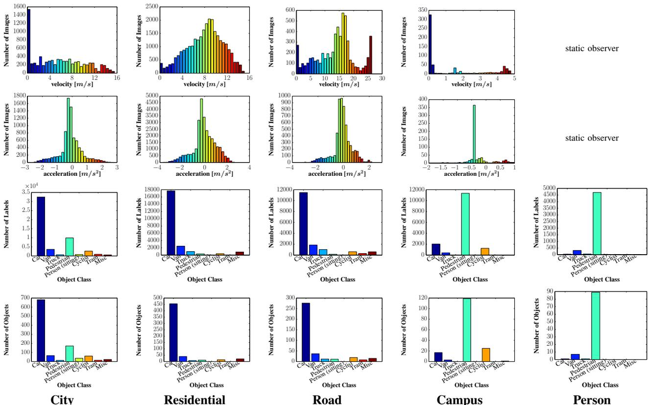
Fig. 11. **Velocities, Accelerations and Number of Objects per Object Class.** For each scene category we show the acceleration and velocity of the mobile platform as well as the number of labels and objects per class. Note that sequences with a purely static observer have been excluded from the velocity and acceleration histograms as they don't represent driving behavior. The category 'Person' has been recorded from a static observer.
