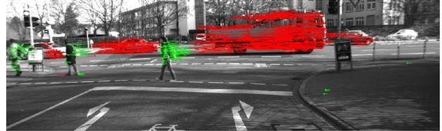
(b) Feature tracking (5 frames, static camera)
