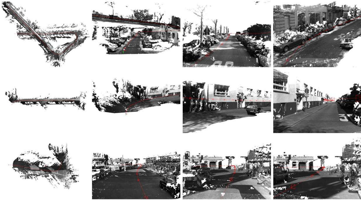
Fig. 8. **Inner-city stereo scans.** Four rendered views (columns) are shown for three sequences (rows). Also see videos at: [www.cvlibs.net](http://www.cvlibs.net)
