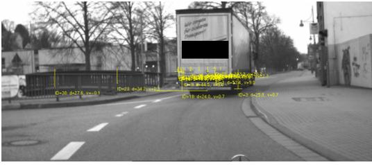
(a) Radar object hypotheses. Each radar object hypothesis marked by a flipped, yellow T symbol can define the full parameter vector defined in equation 4. The BIC permits inferring the actual number of objects in the scene, rejecting the phantom hypotheses.
