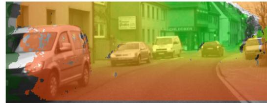
(b) SGM [15] stereo image. The distance is color encoded ranging from red (close) to green (far away).
