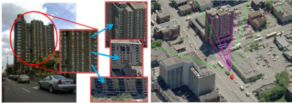
Figure 9: Online processing of a SV image from Panoramio. Extracted and rectified facade returns these top three matching facades from the database. Using the top match, we estimate the camera pose (the point with the emanating rays) and compare it with the ground-truth location (red circle).
