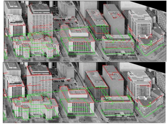
Figure 6: Effect of Graph-Cuts Optimization. The green edges are the SAT edges directly projected to this view and they lie in the ground plane. The red edges are the estimated building top edges. The top row shows the estimates obtained by picking the maximum score for each edge pixel independently; the bottom row shows these estimates refined by the GC optimization.
