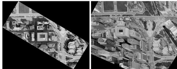
Figure 3: SAT image rotated to align city-block direction with the x-axis (left) and the corresponding BEV image automatically aligned to the SAT image w.r.t the ground-plane using the geo-coordinate information (right).
