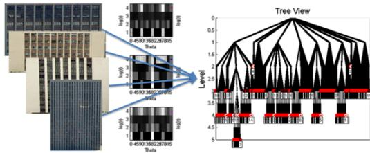
Figure 8: Self-similarity descriptor features extracted from various facades get pushed into an ADT data-structure.
