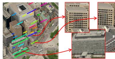
Figure 4: Example of the facade extraction process. a) detected building tops and bottoms, and b) extracted facade tiles.
