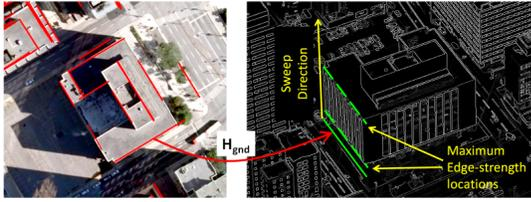
Figure 5: Building top search. Line segments extracted from the SAT imagery are projected to the canny edge map of BEV where a sweep along the gravity direction is expected to give a maximal point at the top edge of the building.
