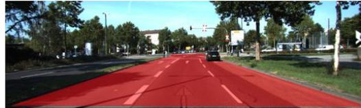
Fig. 1: Sample image with the annotated drivable road area. Note that out of the two parallel road in the image only one is labeled as drivable. Also, the road region occluded by the car is not labeled as drivable.
