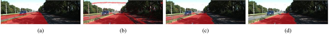
Fig. 4: (a) Initial labeling using OpenStreetMap. (b) Label Refinement using K-Means. (c) Improved Labeling after restricting the allowed road pixels. (d) Final Labeling after removing the non-drivable parallel road.
